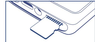
The Solar Bible Bus can also play audio from a properly formatted microSD card. With the player facing you, insert a card with the brass contacts of the card showing face up until it locks in place.
